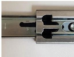
**STEP 2:** Turn the slides over & extend them fully until you can see the black disconnect lever. Pinch it in the direction of the arrow.
